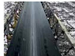
Low rolling resistance belt increases energy efficiency, market entry planned for 2012
