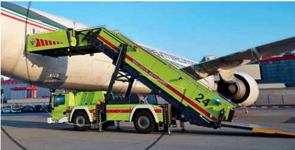
The new E5000 rescue staircase was delivered to Geneva Airport in late 2014. The E5000 completes Rosenbauer's fleet of rescue staircase vehicles. It covers heights of between 2.50 m and 5.50 m.
