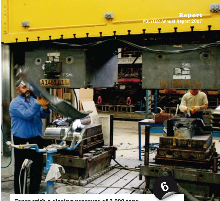
Press with a closing pressure of 2,000 tons Slowly, our spoiler is beginning to take shape.
