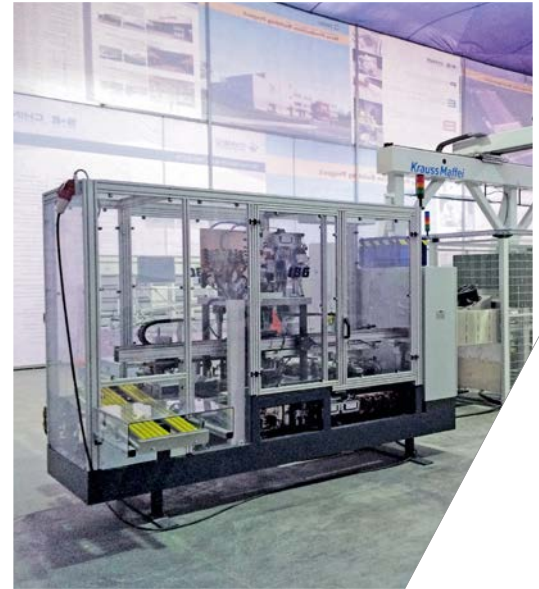
One of three fully automatic injection moulding lines with integrated testing system for the production of transmission oil pans.
