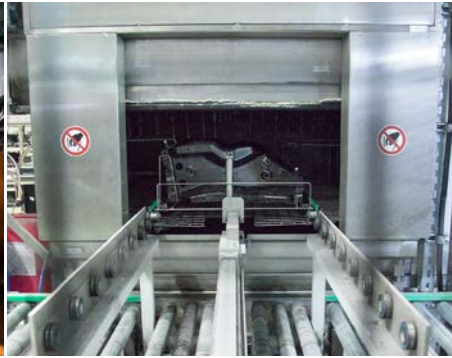
In the automatic washing unit, the component is freed from carbon dust and dried ...
