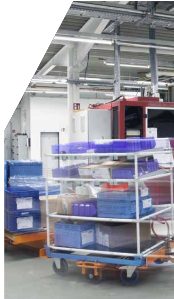
A train carrying purchased and semi-finished parts runs along a clearly defined route in a two-hour rhythm, thus reducing the logistical distances as compared to supply by forklift.
