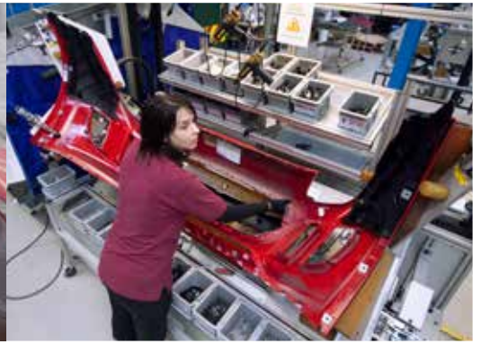
1,000 different bumper variations demand a complex technical control system that supports the employees at the POLYTEC location in Bromyard during the assembly process.
