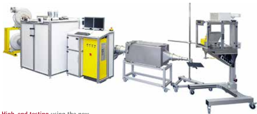
High-end testing using the new air filter system test stand in Lohne
