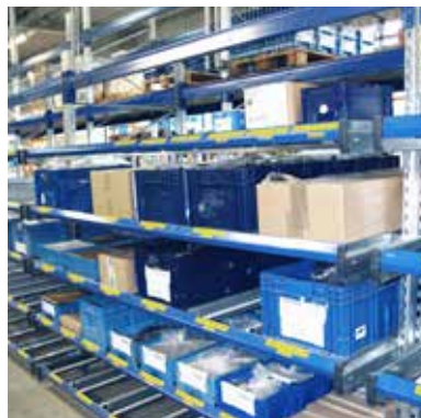
The "marketplace" serves as an interface between production and warehousing. It stocks all the components necessary for the continual supply of the hot gas welding area.
