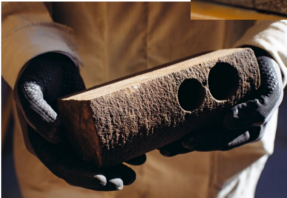
This section of a core from the TECH Center & Lab's archives was drilled in 1958 in Austria. The lab has collected a vast store of cores in its 40 years of existence (top). The holes in this oil-stained cross section of a core originate from previous sample extractions for porosity measurements (left).
