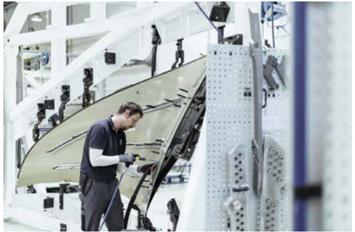
Manufacture of a winglet for the A350-900 at the mixed model line
