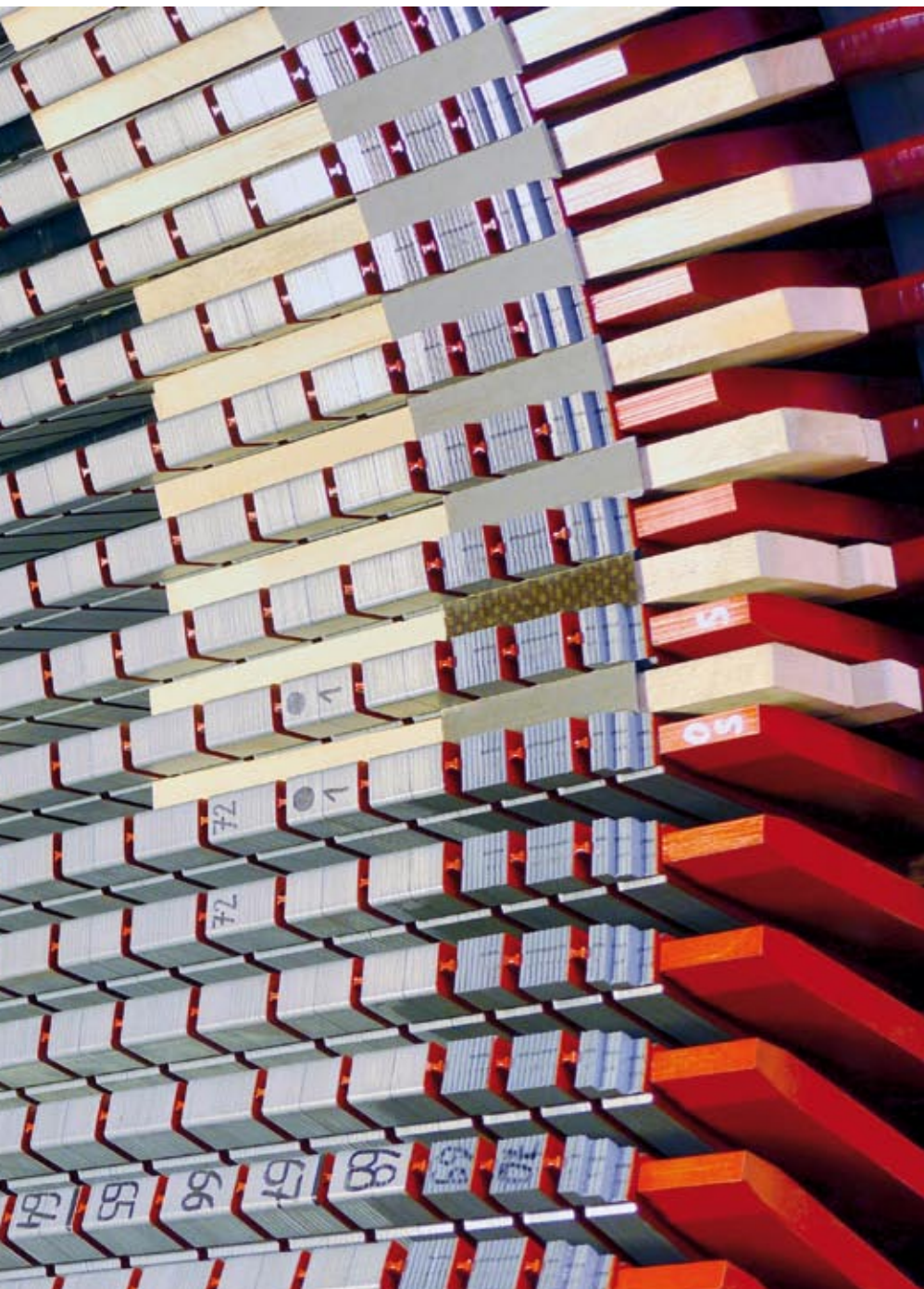
▲ Part of a turbo generator which is used in gas and steam power stations.
