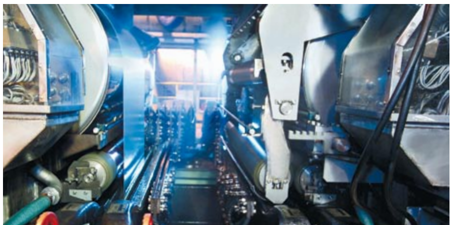
▲ Inside of a Gravitel cell, where zinc is deposited electrolytically onto the steel strip.
