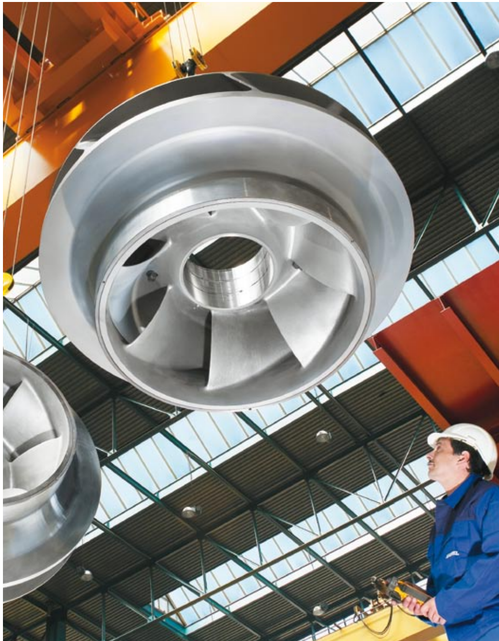
▲ Two impellers manufactured for a spiral casing pump used in the irrigation of farmland in India.
