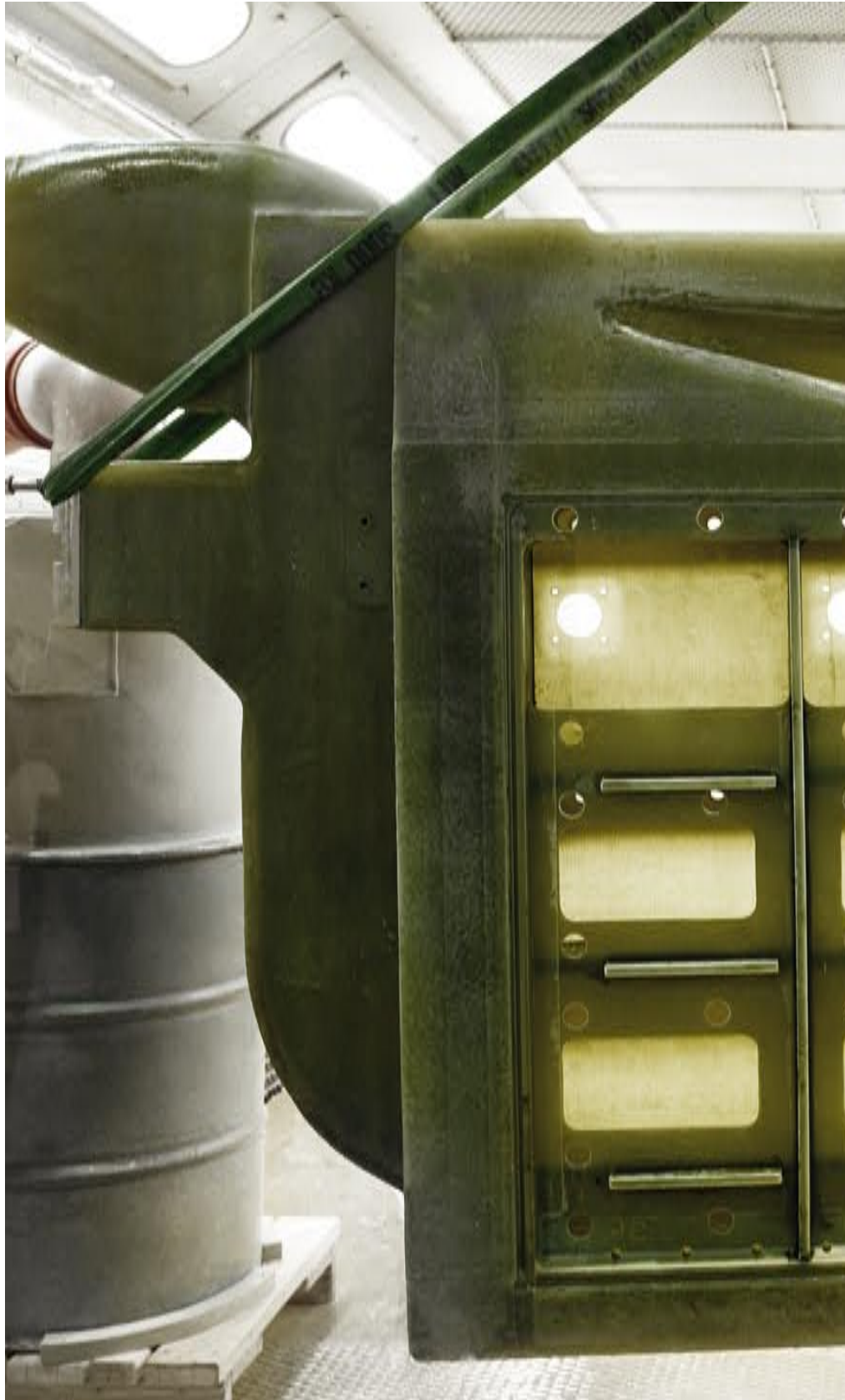
Gravitel anode box for electrolytic galvanizing plants: ANDRITZ METAL's Gravitel process ASD is used in the production of top quality electro-galvanized steel strip for the automotive and household appliances industries. ▶
