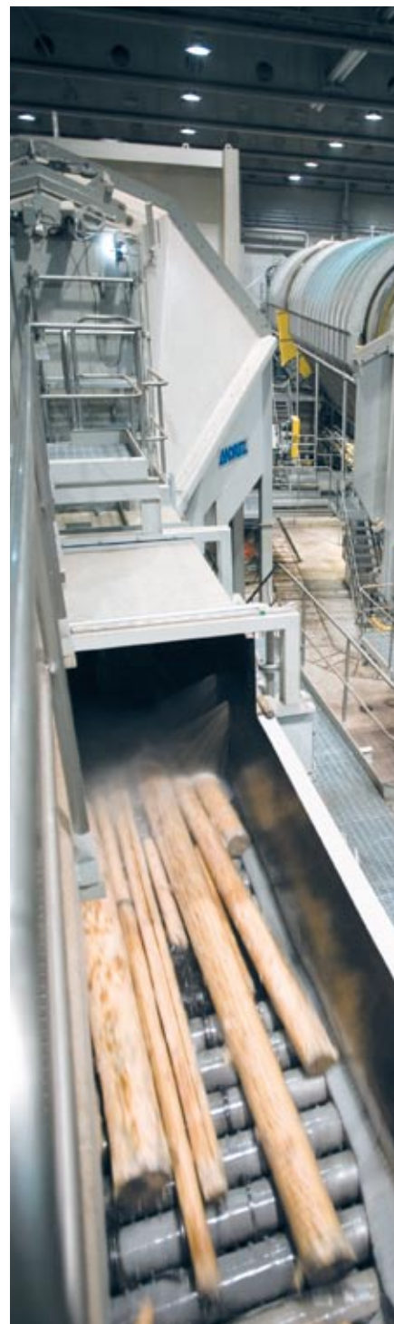
▲ ANDRITZ debarking drums are used to debark and wash logs for pulp production.
