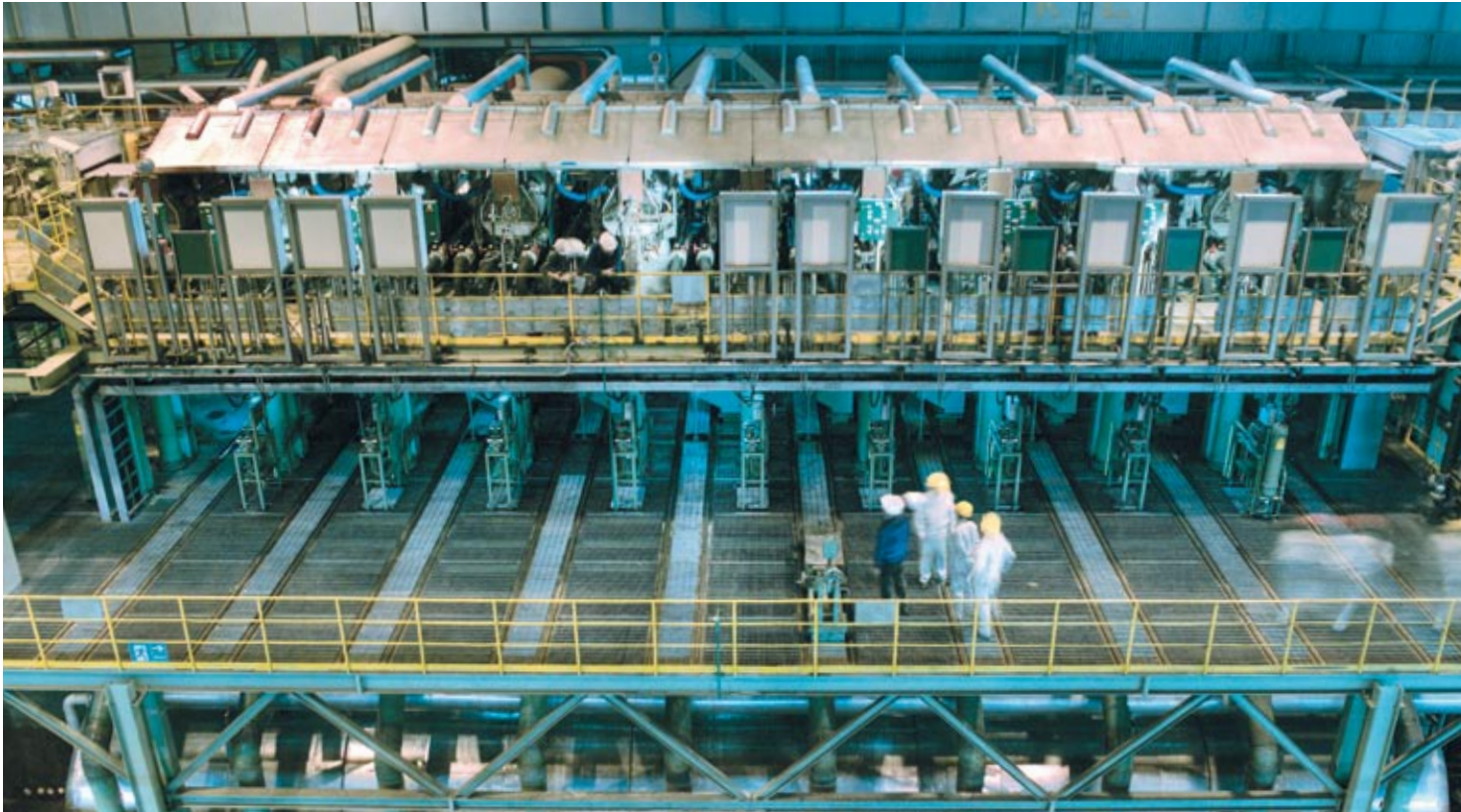
▲ Galvanizing section of the electrolytic galvanizing line supplied by ANDRITZ METALS to Baosteel, Shanghai, China. The line is based on the Gravitel process and started operation in December 2008.
