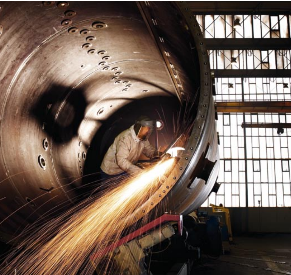
▲ Key process equipment for ANDRITZ plants and products is manufactured and assembled at ANDRITZ's own workshops. An example is the pressure vessel (shown in the picture) for a hyperbaric filtration plant (HBF ES ) that will be supplied to Anglo Chile for copper suspension filtration. Simple components are purchased from qualified suppliers who are subjected to regular quality checks and on-time performance monitoring.
