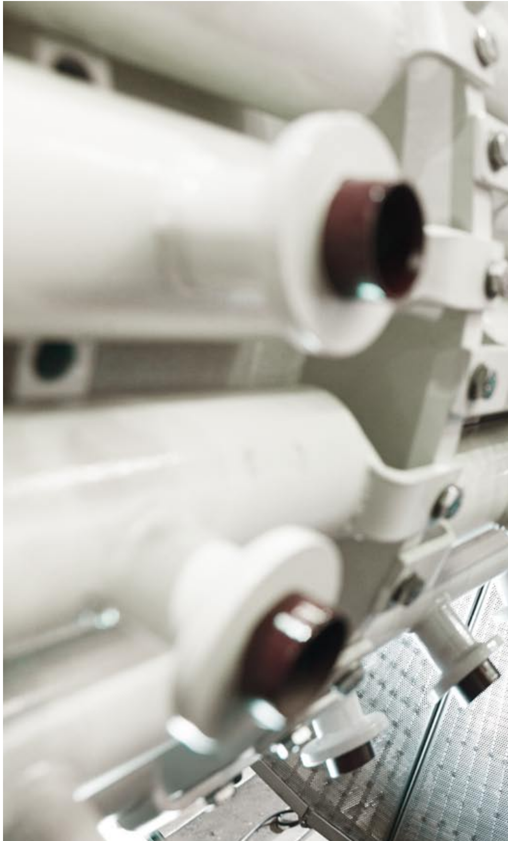
Filter shaft for a vacuum disc filter used in hard coal dressing to obtain coking coal. ▶
