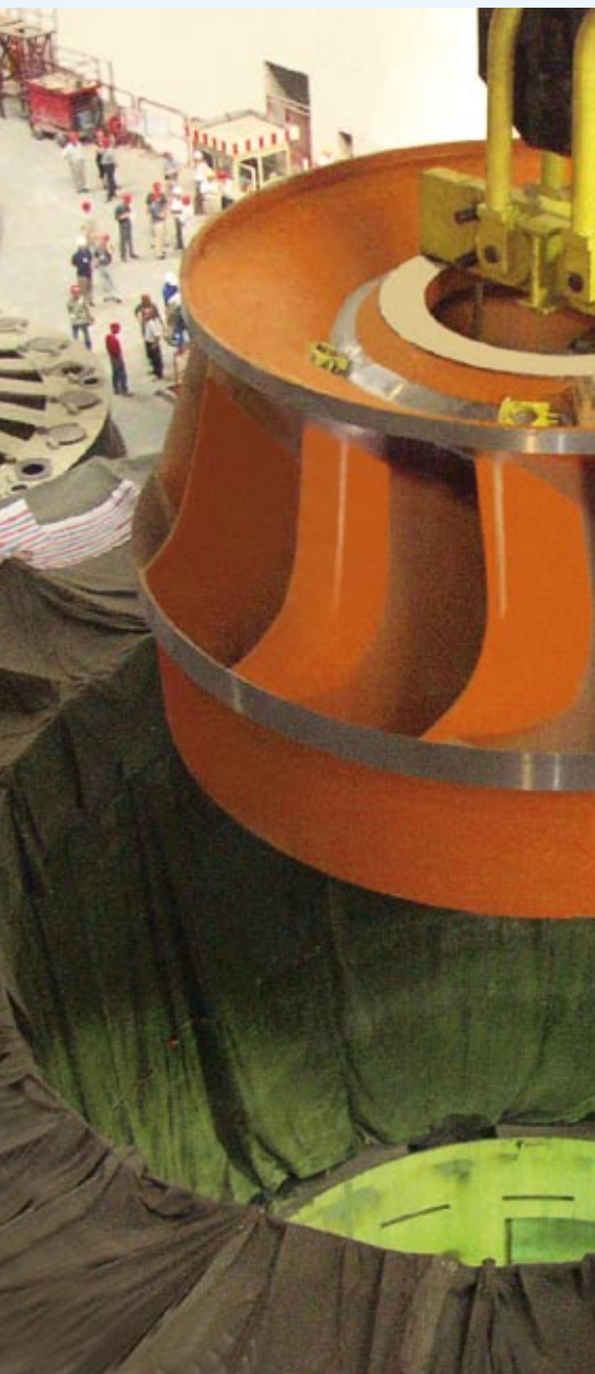
▲ GE Hydro technology: the turbine runner for the Three Gorges dam, China, manufactured by the GE Hydro/Voith Siemens consortium.
