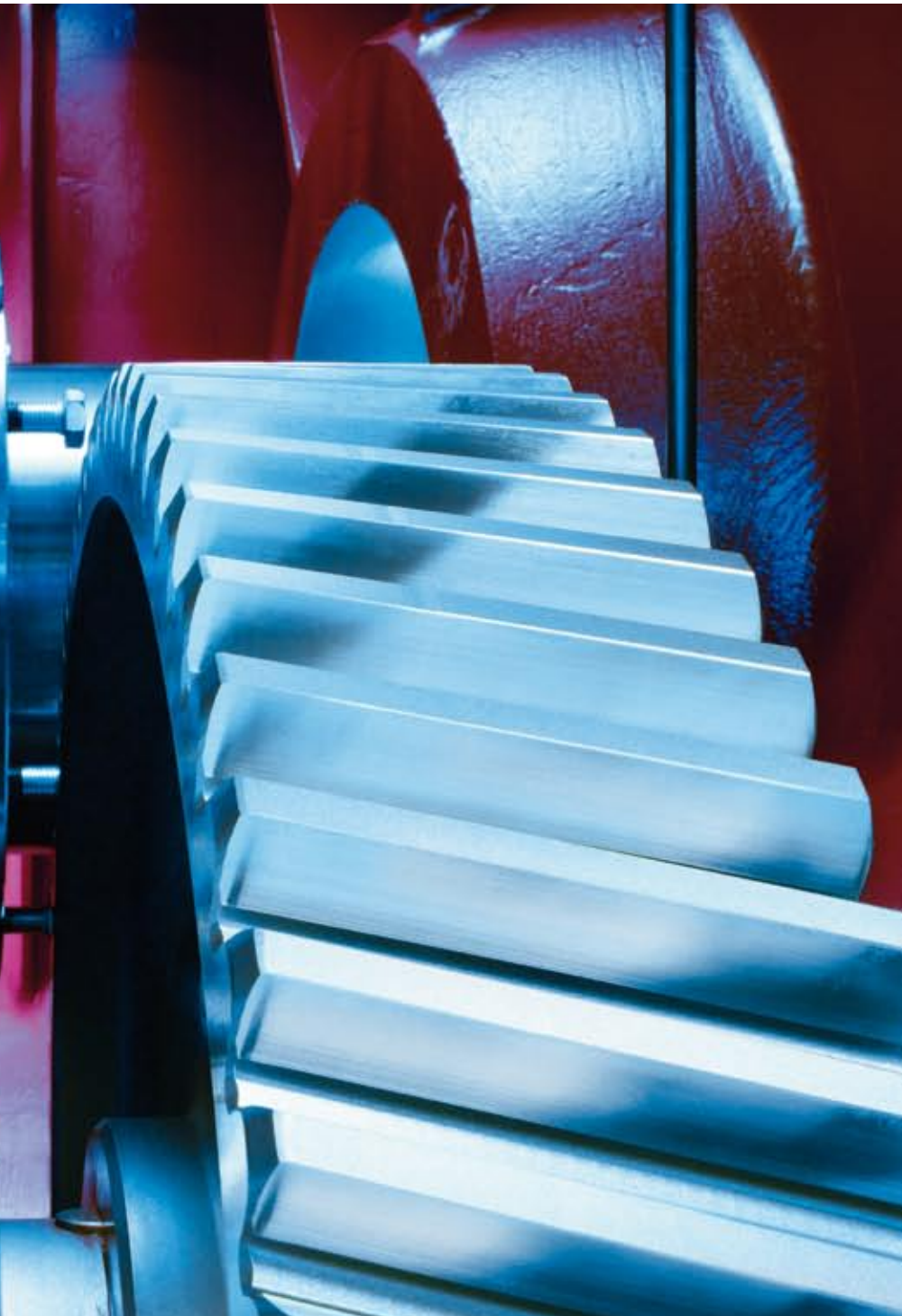
▲ Close-up of an ANDRITZ FEED & BIOFUEL pellet mill for animal feed pelleting. Shown is the gearbox.
