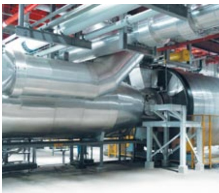
▲ One of the five drying drums supplied by ANDRITZ ENVIRONMENT & PROCESS for the drying plant for PUB (Public Utility Board), Changi, Singapore.
