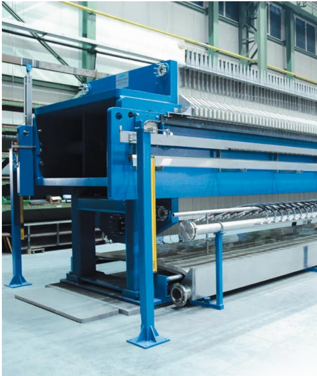
▲ ANDRITZ ENVIRONMENT & PROCESS membrane filter press used to dewater sludge from municipal wastewater treatment plants. The press reduces the sludge volume and produces clear filtrate that can be discharged to the sewer.
