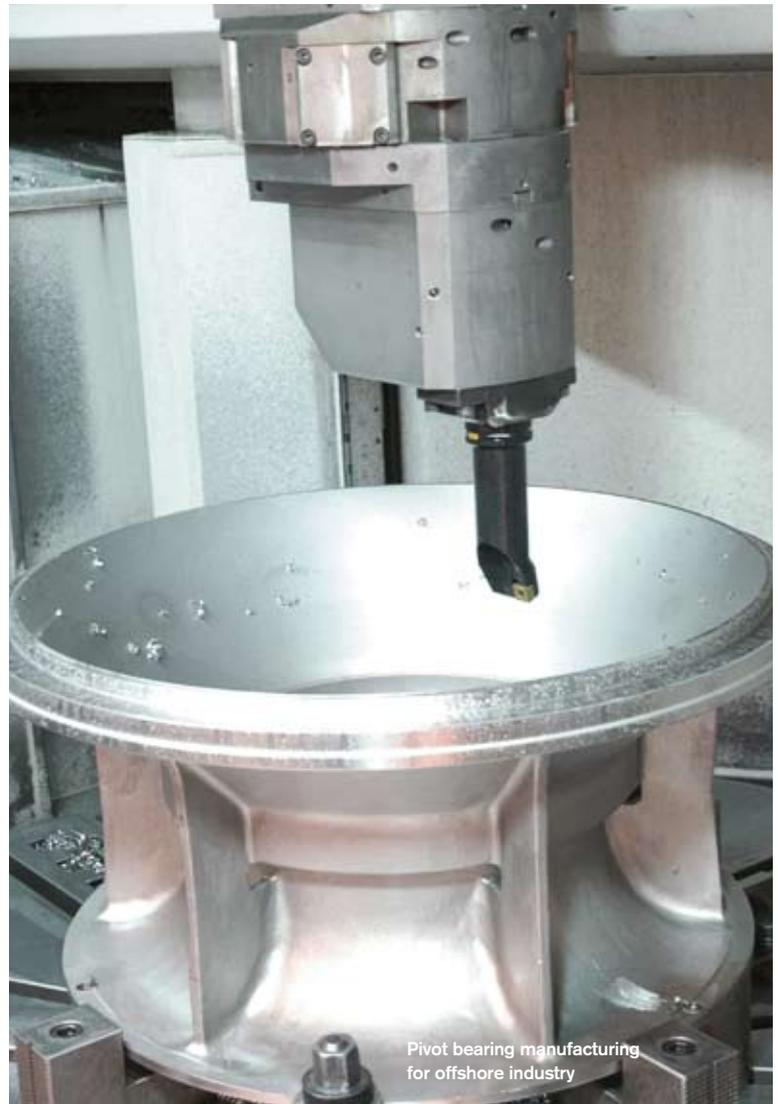
Pivot bearing manufacturing for offshore industry
