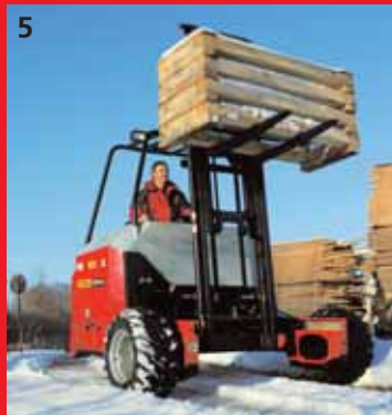
5 Crayler portable forklift 6 Palgate tailgate 7 Telescopic crane 8 Truck-mounted knuckle-boom crane
