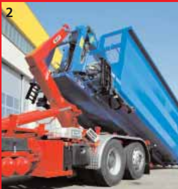
1 Bison aerial work platform 2 Palfit container handling system 3 Epsilon forestry crane 4 High-tech railway application
